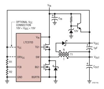
Figure 10c. Secondary Output Loop and  $V_{CC}$  Connnection
