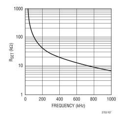
Figure 7. Timing Resistor (R<sub>SET</sub>) Value
