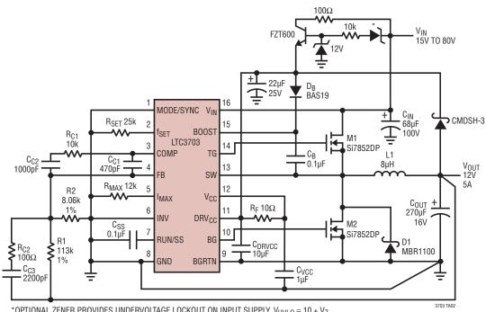
\*OPTIONAL ZENER PROVIDES UNDERVOLTAGE LOCKOUT ON INPUT SUPPLY,  $V_{UVL0} \cong 10 + V_Z$
