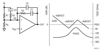
Figure 14. Type 3 Schematic and Transfer Function
