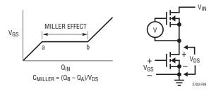
Figure 9. Gate Charge Characteristic
