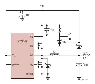
Figure 10a.  $V_{CC}$  Generated from 10V <  $V_{OUT}$  < 15V
