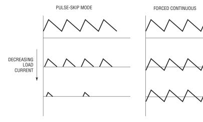
Figure 5. Comparison of Inductor Current Waveforms for Pulse-Skip Mode and Forced Continuous Operation
