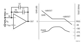
Figure 13. Type 2 Schematic and Transfer Function
