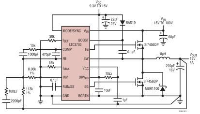
Figure 1. High Efficiency High Voltage Step-Down Converter
