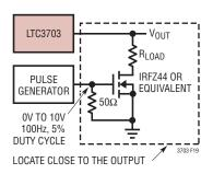
Figure 19. Transient Load Generator
