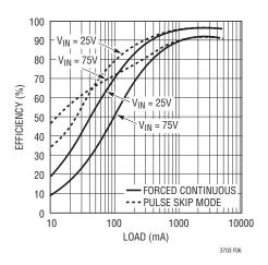
Figure 6. Efficiency in Pulse-Skip/Forced Continuous Modes
