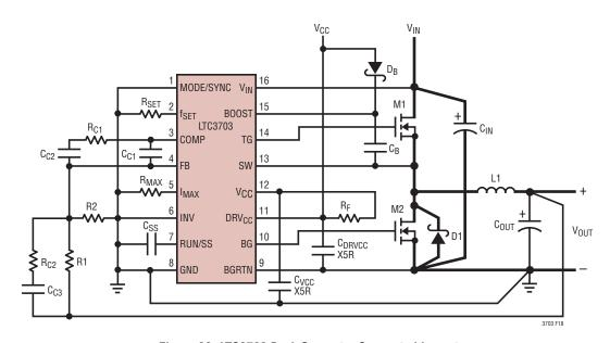
Figure 20. LTC3703 Buck Converter Suggested Layout
