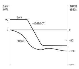
Figure 16. Transfer Function of Boost Modulator
