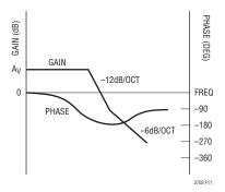
Figure 11. Transfer Function of Buck Modulator
